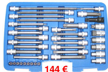
BGS5184 38-delig set - Jeu 38 pièces 1/4 TS10-TS20 / 1/2 RIBE 7x240-8x240 9x100-10x140 / 1/2 TX40-->TX70x140 1/2 IN7-10-11-13x140 + 14-->24 x55mm XZN 9x100+10-12-14x140+16x55-16x100 XZN 18 - TX80x100 - TTX30x300-INB5x160
